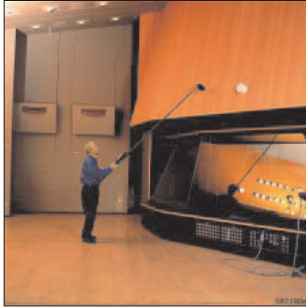
Fig. 16 Mapping the sound reduction to find leakages between studio and control room
